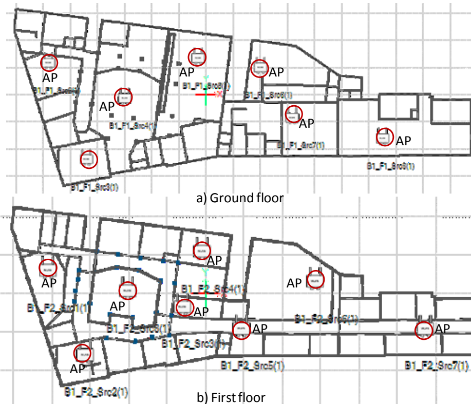
Figure 12 WLAN AP deployment randomly
